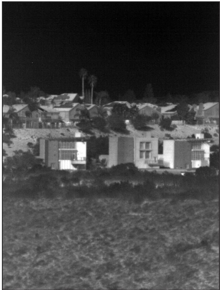
Targets at approximately 1 km imaged from the Canyon View Cleanroom at MSSS with VNFOV optics. Image has been 1-point non-uniformity corrected using an image taken with the internal shutter actuated. Image Credit: MSSS
